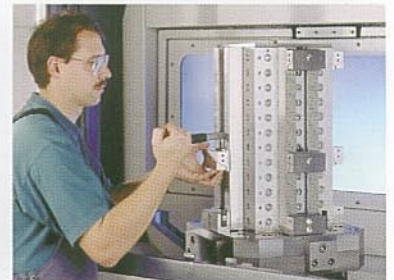
3. The clamping module is fixed by means of the eccentric screw and the torque wrench 50 - 70 Nm.
