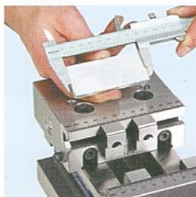
Install the base jaw. The blank is approx. 2 mm larger than the finished workpiece.
