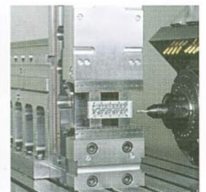
SlimFlex jaw system: optimum 3-side machining.
